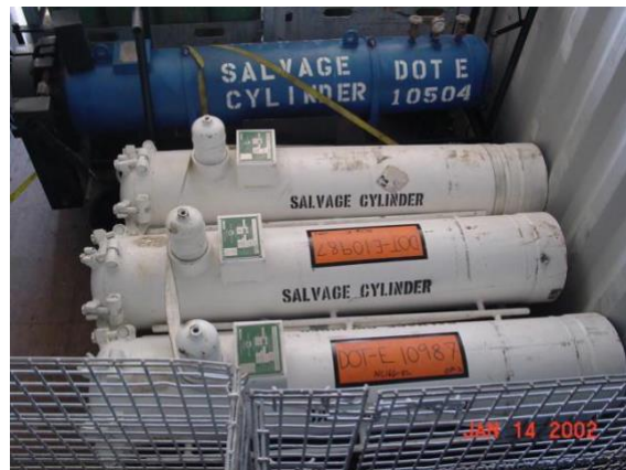
Damaged cylinders placed in over packs during emergency response, Puerto Rico Public Works Authority.
